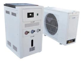
The indoor unit is consist of water pump, water reservoir and evaporator while the outdoor unit consist of compressor, fan and condenser, which can discharge all heat and noise outside. Split type design improve comfort and reduce the noise, at the same time enhance the cooling capacity. Their large refrigeration capacity with steady operation also used as a central supply of cooling water for labs or complete buildings.
